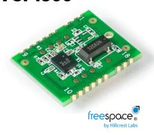
The FSM300 is a self-contained AHRS/IMU module integrating a 3-axis accelerometer, 3-axis gyroscope, and 3-axis magnetometer, along with a low-power 32-bit ARM Cortex M0+ MCU running Hillcrest's high-performance sensor hub software stack.
