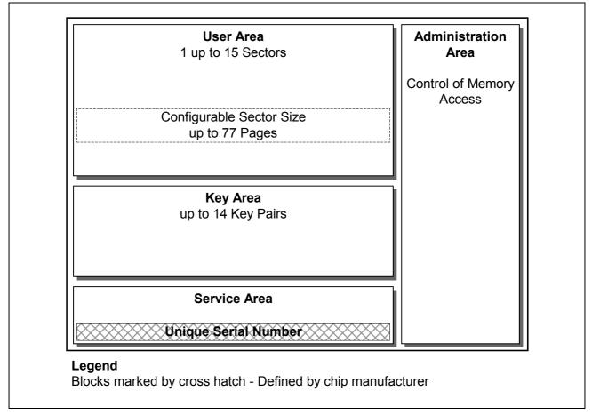
Figure 3 Memory principle of SLE 55R04
