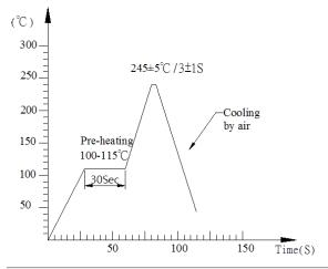
Recommendable wave soldering condition is as follows: Note 1: It is requested that reflow soldering should be executed after heat of product goes down to normal temperature. Note 2: Peak reflow temperature of 250°C maximum of 10 seconds, with a maximum duration of 40-60 seconds between 220°C and 250°C
