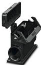
Box mounting bases B24, with single locking latch, material: PA, protective cover material: PA, cable outlets: 2, lateral, height: 84 mm, cable gland: none, support sleeve: no, 2x M32, protective cover: yes, Standard, including 2x reducing adapter
