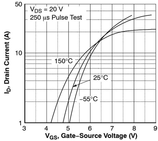
Figure 2. Transfer Characteristics
