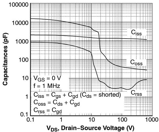
Figure 5. Capacitance Characteristics
