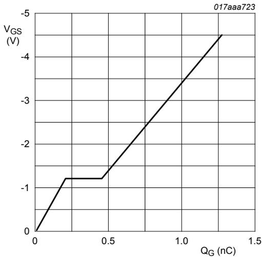
$I_D = -0.3$  A;  $V_{DS} = -10$  V;  $T_{amb} = 25$  °C
