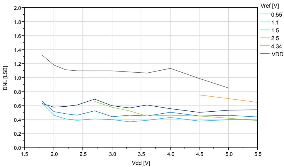
**Figure 38-44. ATtiny1614/1616/1617: REFSEL = Internal reference, DNL vs.  $V_{REF}$  ( $V_{DD}=5.0V$ ,  $f_{ADC}=115ksps$ )**
