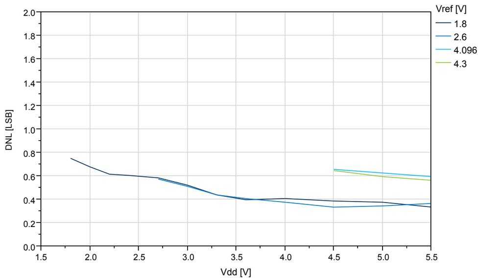
**Figure 38-54. ATtiny1614/1616/1617 REFSEL = External reference, DNL vs.  $V_{REF}$  ( $V_{DD}=5.0V$ ,  $f_{ADC}=115kps$ )**
