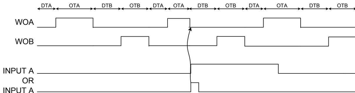
If Input mode 8 is used on input B and an positive input event occurs while in On time B, the TCD counter jumps to Dead time A.
