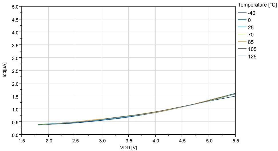
**Figure 38-37. ATtiny1614/1616/1617: BOD Current vs. V<sub>DD</sub> (Sampled BOD at 1kHz)**
