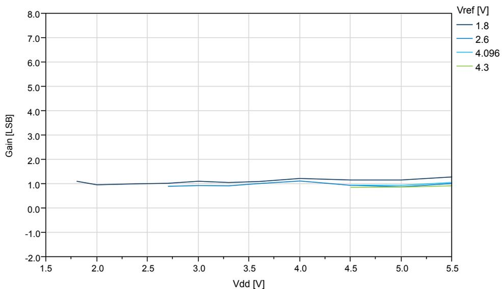
**Figure 38-56. ATtiny1614/1616/1617 REFSEL = External reference, Gain vs.  $V_{REF}$  ( $V_{DD}=5.0V$ ,  $f_{ADC}=115ksps$ )**
