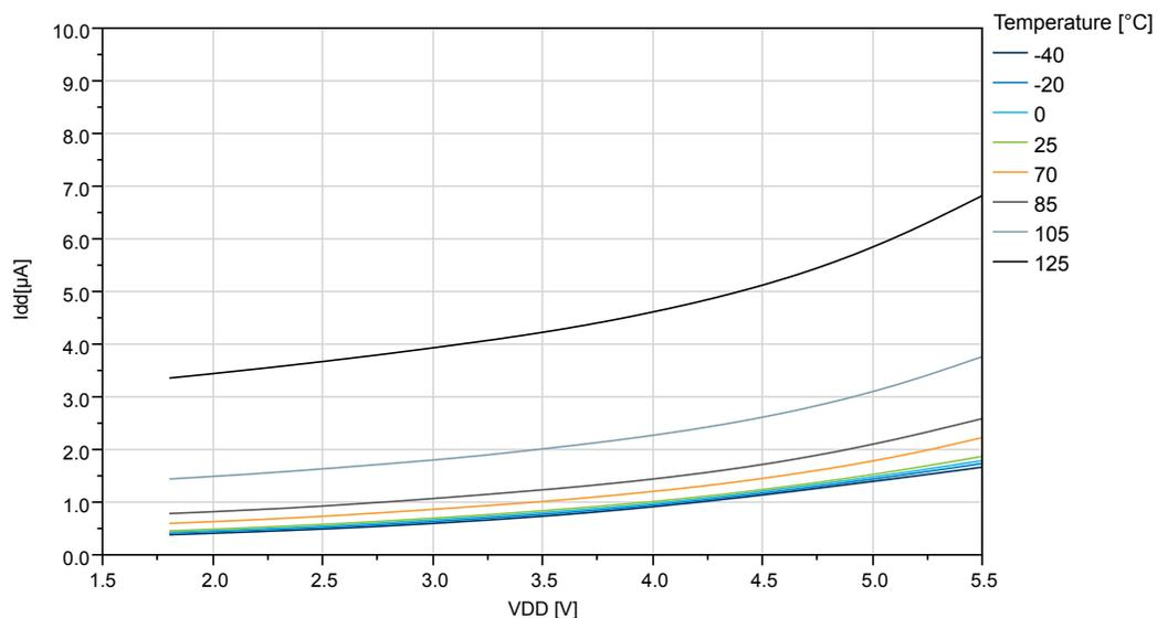
**Figure 38-15. ATtiny1614/1616/1617: Standby Mode Supply Current vs.  $V_{DD}$  (Sampled BOD running at 1kHz)**
