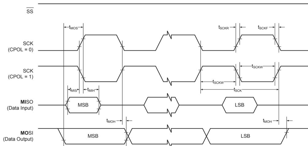
**Figure 37-4. USART in SPI Mode - Timing Requirements in Slave Mode**
