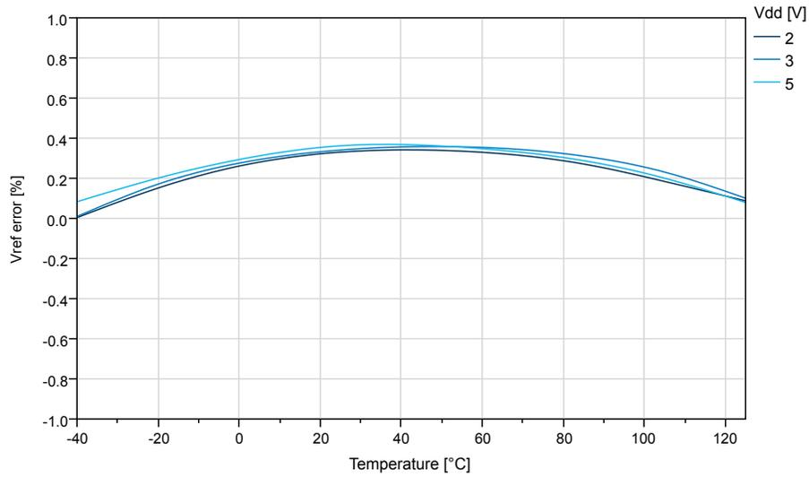
Figure 38-32. ATtiny1614/1616/1617: Internal 1.1V Reference vs. Temperature
