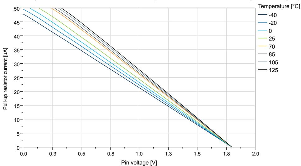
**Figure 38-29. ATtiny1614/1616/1617: IO Pin Pull-Up Resistor Current vs. Input Voltage ( $V_{DD}=3.0V$ )**
