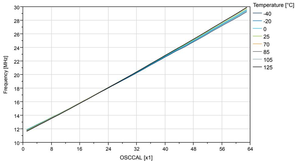
**Figure 38-67. ATtiny1614/1616/1617: OSC20M Internal Oscillator: Frequency vs. Temperature**
