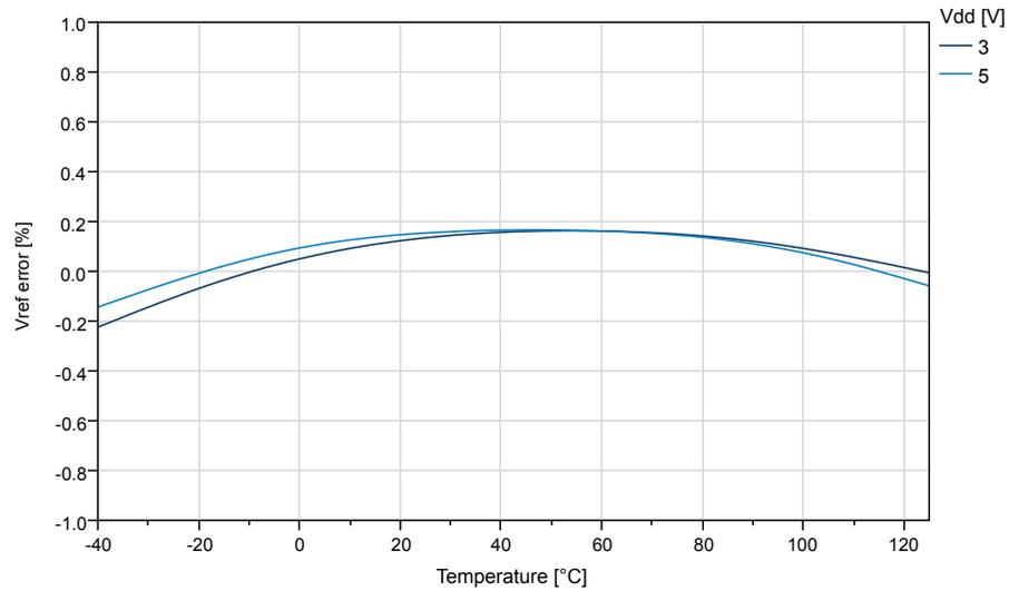
**Figure 38-34. ATtiny1614/1616/1617: Internal 4.34V Reference vs. Temperature**
