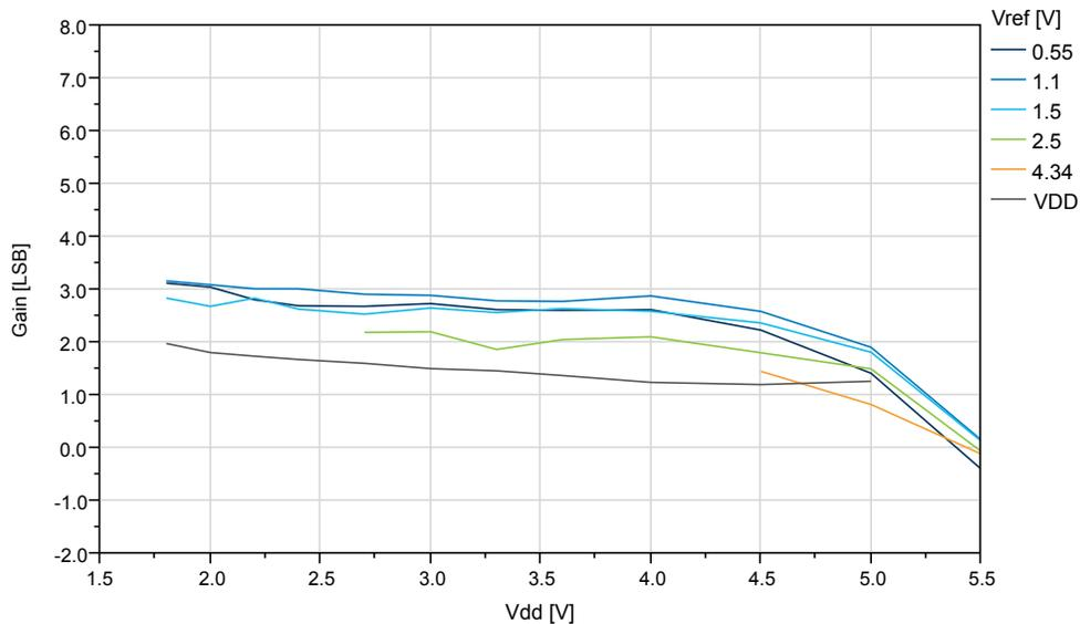
**Figure 38-46. ATtiny1614/1616/1617: REFSEL = Internal reference, Gain Error vs.  $V_{REF}$  ( $V_{DD}=5.0V$ ,  $f_{ADC}=115kps$ )**
