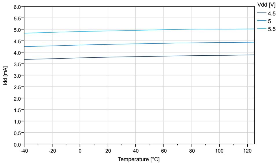
**Figure 38-9. ATtiny1614/1616/1617: Idle Supply Current vs.  $V_{DD}$  ( $f=32\text{KHz OSCULP32K}$ )**
