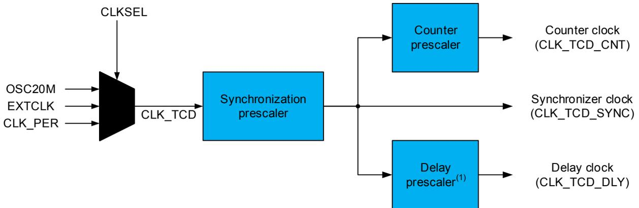
1. Used by input blanking/delay event out
