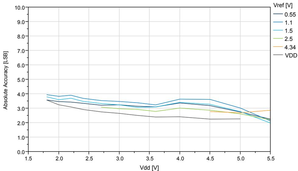
**Figure 38-42. ATtiny1614/1616/1617: REFSEL = Internal reference, Absolute Accuracy vs.  $V_{REF}$  ( $V_{DD}=5.0V$ ,  $f_{ADC}=115kps$ )**
