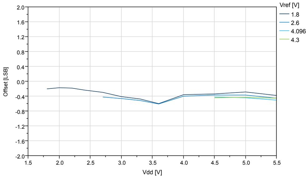
**Figure 38-60. ATtiny1614/1616/1617 REFSEL = External reference, Offset vs.  $V_{REF}$  ( $V_{DD}=5.0V$ ,  $f_{ADC}=115ksps$ )**
