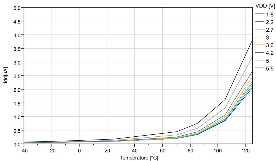
**Figure 38-11. ATtiny1614/1616/1617: Power Down Mode Supply Current vs.  $V_{DD}$  (all functions disabled)**
