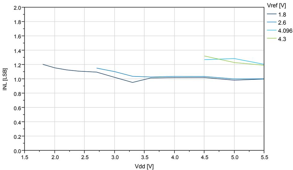
**Figure 38-58. ATtiny1614/1616/1617 REFSEL = External reference, INL vs.  $V_{REF}$  ( $V_{DD}=5.0V$ ,  $f_{ADC}=115kpsps$ )**
