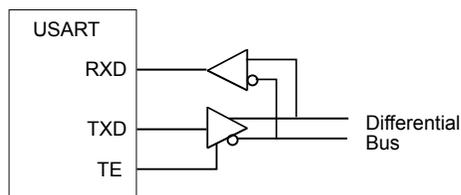
The TE pin goes high one baud clock cycle in advance of data being shifted out, to allow some guard time to enable the external line driver. The TE pin will remain high for the complete frame including stop bit(s).
