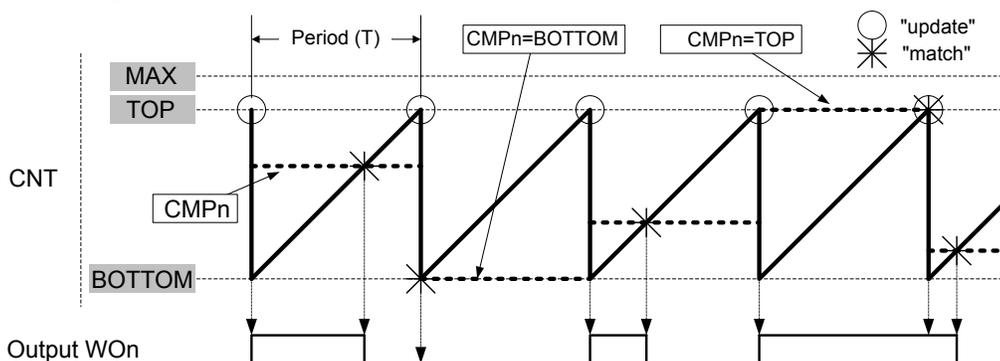
The TCA.PER register defines the PWM resolution. The minimum resolution is 2 bits (TCA.PER=0x0003), and the maximum resolution is 16 bits (TCA.PER=MAX).
