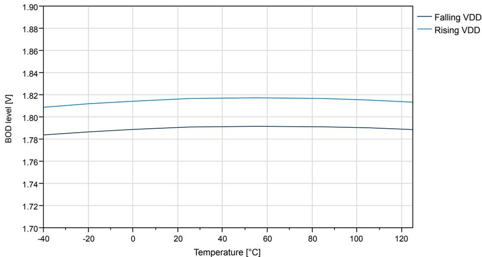
**Figure 38-39. ATtiny1614/1616/1617: BOD Threshold vs. Temperature (Level 2.6V)**
