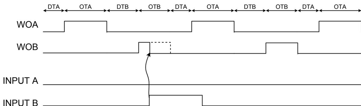
**Input Mode 10: Stop Output on Edge, Maintain Frequency**
