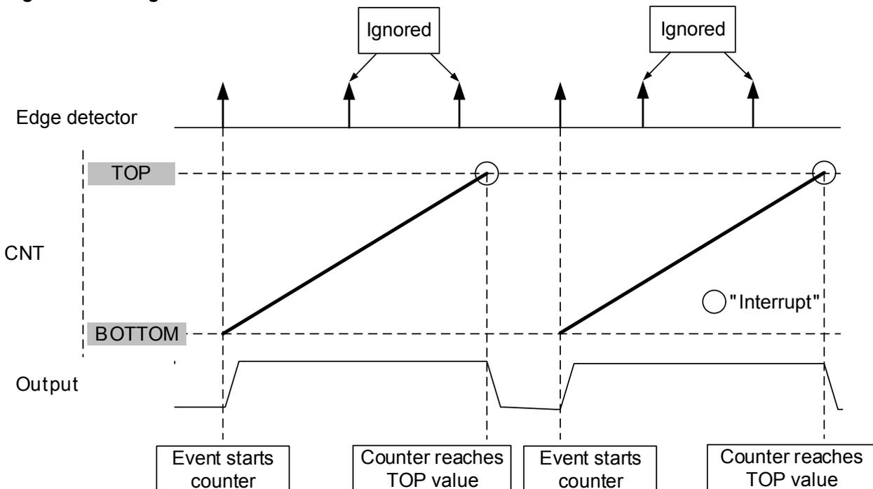
If the ASYNC bit in TCB.CTRLB is '0', the event pulse needs to be longer than one system clock cycle in order to guarantee edge detection.
