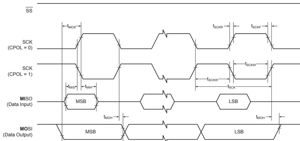
**Figure 37-6. SPI - Timing Requirements in Slave Mode**
