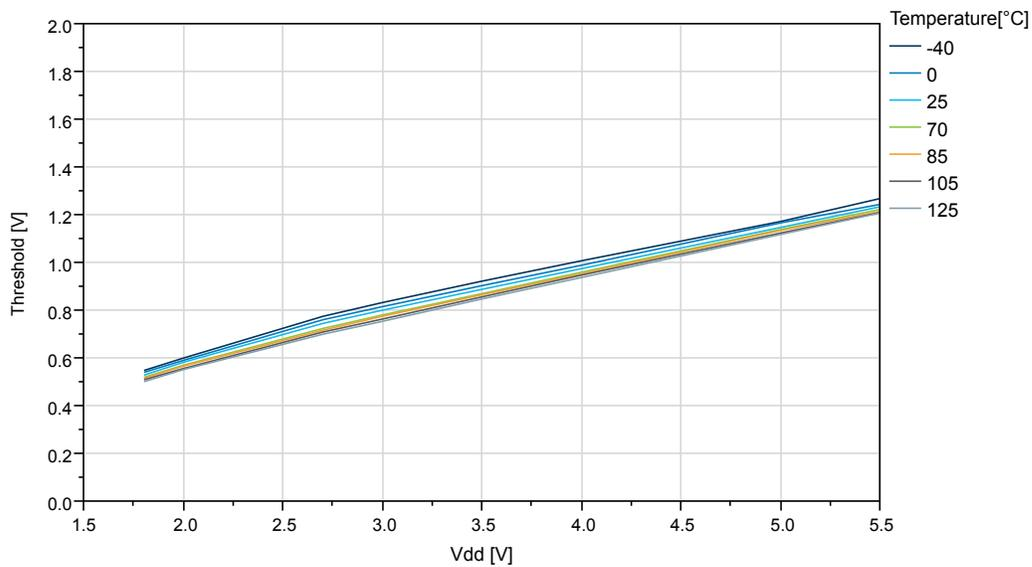
**Figure 38-17. ATtiny1614/1616/1617: IO Pin Input Threshold Voltage vs.  $V_{DD}$  ( $T=25^{\circ}\text{C}$ )**
