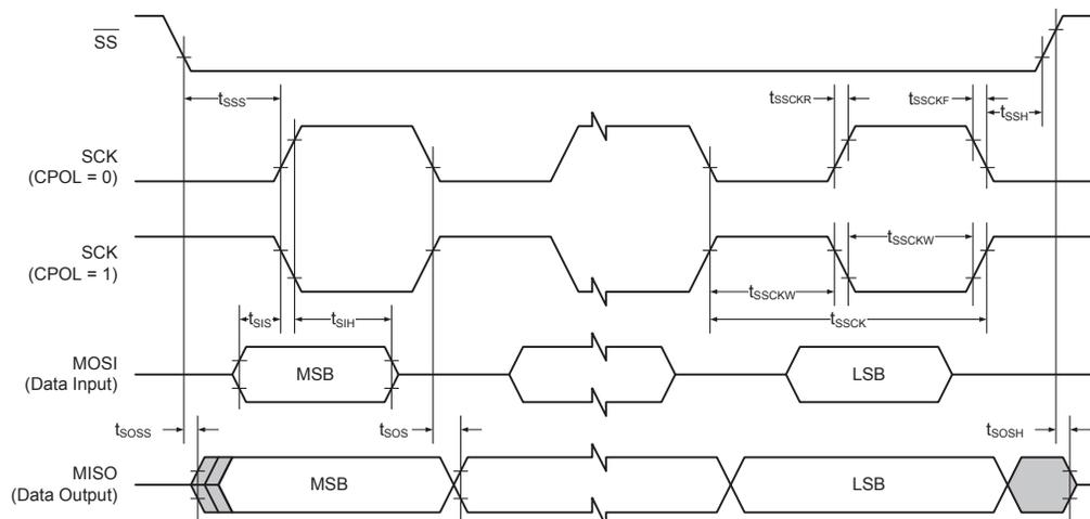
**Table 37-16. USART in SPI Mode - Timing Characteristics**
