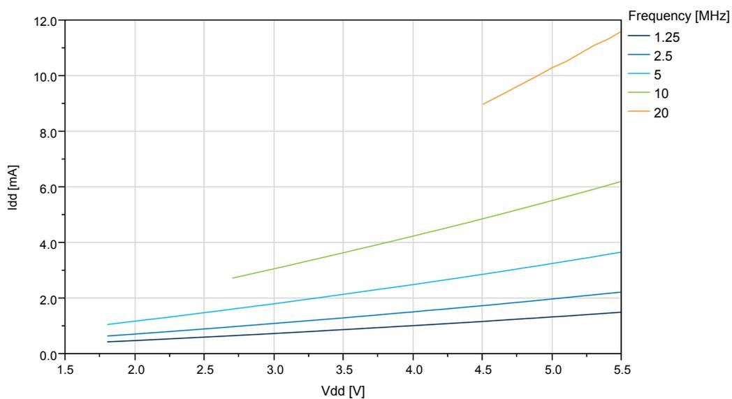
**Figure 38-5. ATtiny1614/1616/1617: Active Supply Current vs.  $V_{DD}$  ( $f=32\text{KHz OSCULP32K}$ )**
