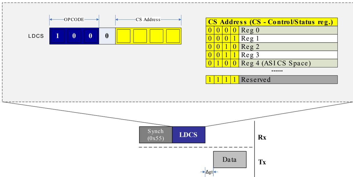
The Figure above shows a typical example of `LCDS` data transmission. A data byte from the `LCDS` space is transmitted from the UPDI after the Guard-Time is completed.
