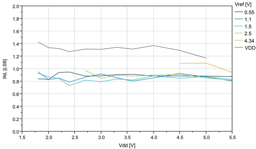
**Figure 38-48. ATtiny1614/1616/1617: REFSEL = Internal reference, INL vs.  $V_{REF}$  ( $V_{DD}=5.0V$ ,  $f_{ADC}=115ksps$ )**
