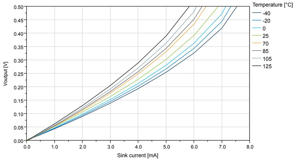
**Figure 38-21. ATtiny1614/1616/1617: IO Pin Output Voltage vs. Sink Current ( $V_{DD}=3.0V$ )**
