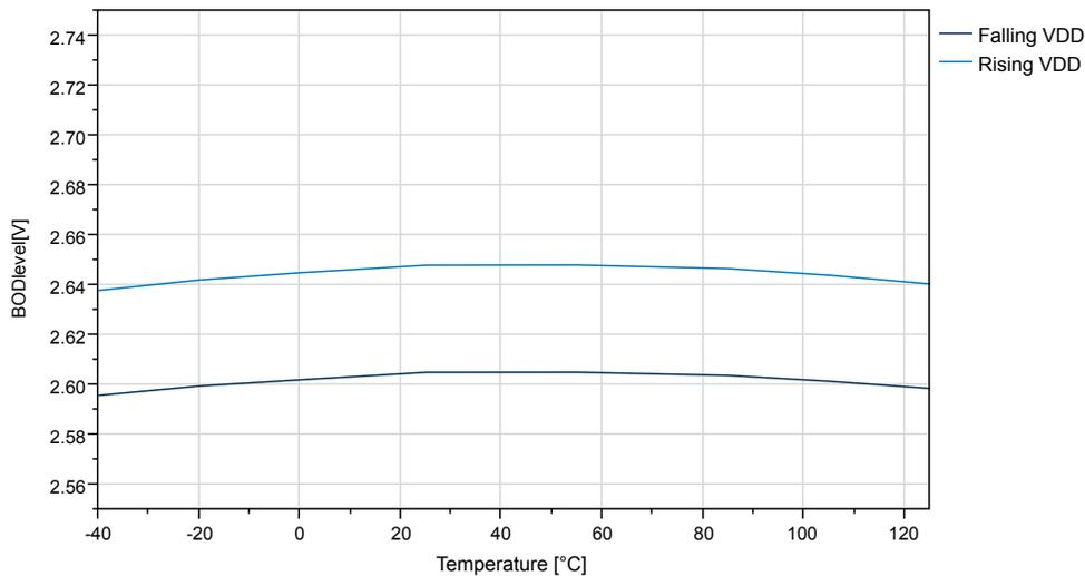
**Figure 38-40. ATtiny1614/1616/1617: BOD Threshold vs. Temperature (Level 4.3V)**
