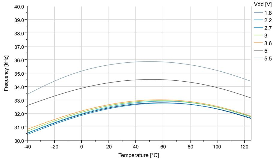
Figure 38-70. ATtiny1614/1616/1617: OSCULP32K Internal Oscillator Frequency vs. V<sub>DD</sub>
