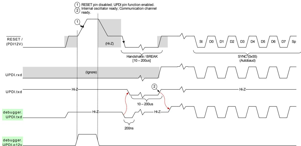
When enabled by 12V, only a POR will disable the UPDI configuration on the  $\overline{\text{RESET}}$  pin, and restore the default setting. If issuing a UPDI disable command through the UPDIDIS bit in UPDI.CTRLB, the UPDI will be reset and the clock request will be canceled, but the  $\overline{\text{RESET}}$  pin will remain in UPDI configuration.
