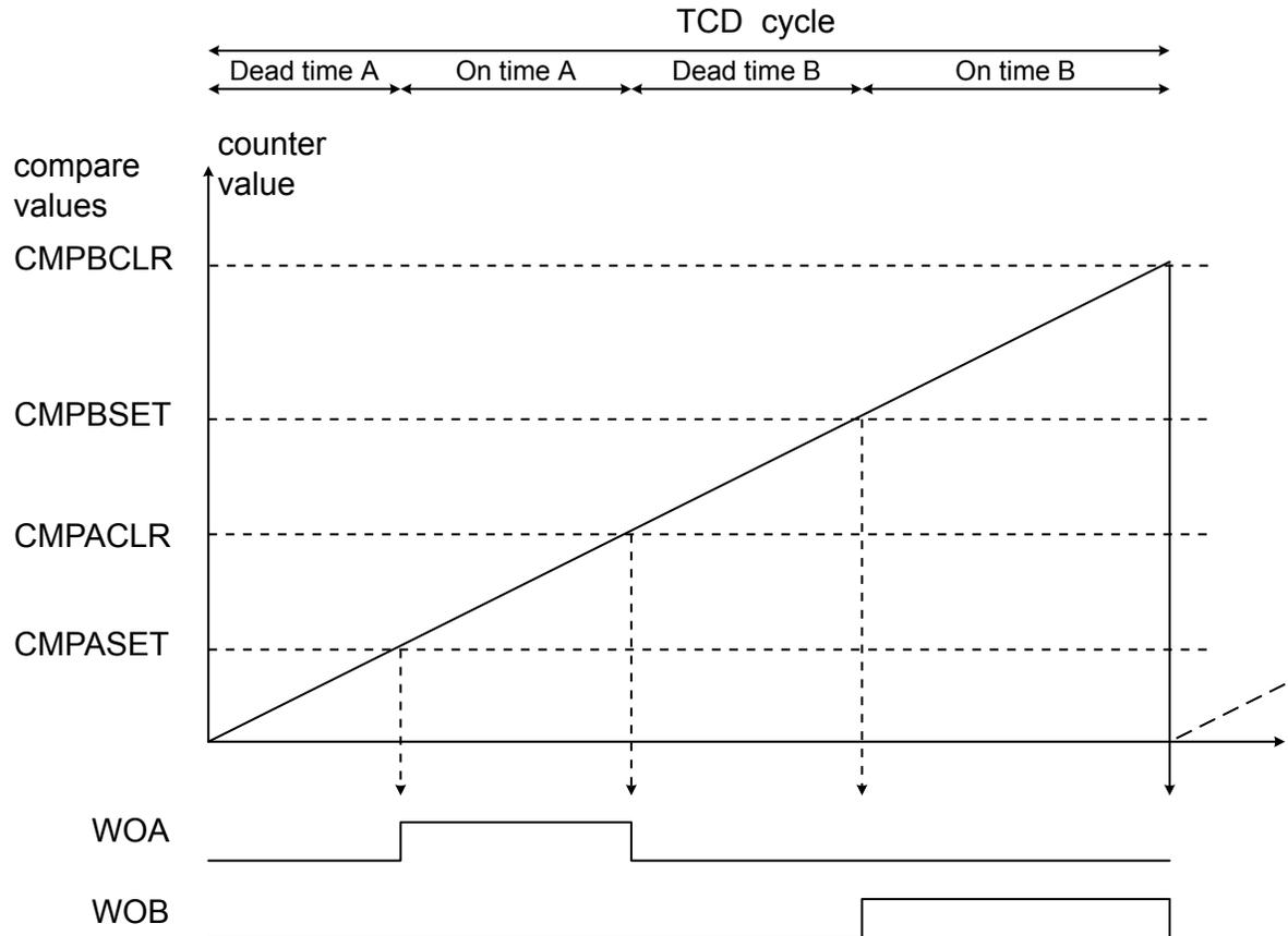
In the figure above,  $CMPASET < CMPACLR < CMPBSET < CMPBCLR$ . This is required in One Ramp Mode to avoid overlapping outputs. The figure below is an example where  $CMPBSET < CMPASET < CMPACLR < CMPBCLR$ , resulting in an overlap of the outputs.
