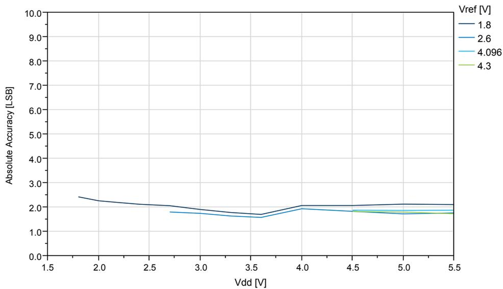
**Figure 38-52. ATtiny1614/1616/1617 REFSEL = External reference, Absolute Accuracy vs.  $V_{REF}$**
