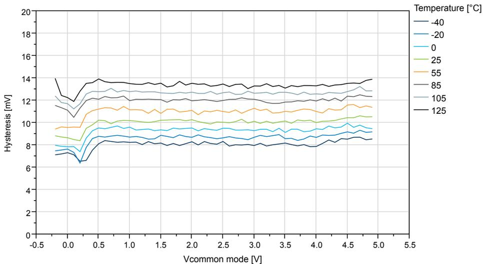
**Figure 38-62. ATtiny1614/1616/1617: Hysteresis vs.  $V_{CM}$  - 10mV to 50mV ( $V_{DD}=5V$ ,  $T=25^{\circ}C$ )**
