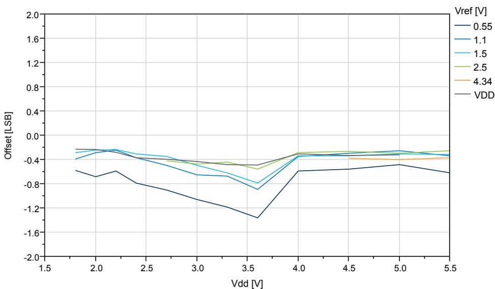
**Figure 38-50. ATtiny1614/1616/1617: REFSEL = Internal reference, Offset Error vs.  $V_{REF}$  ( $V_{DD}=5.0V$ ,  $f_{ADC}=115kpsps$ )**
