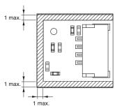
Note: Due to insulation distance limitations, do not allow metal parts to come into contact with the Sensor.
