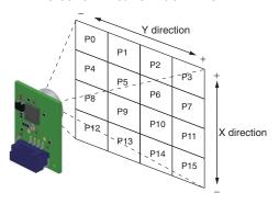
Note: Definition of view angle: Using the maximum Sensor output as a reference, the angular range where the Sensor output is 50% or higher when the angle of the Sensor is changed is defined as the view angle.
