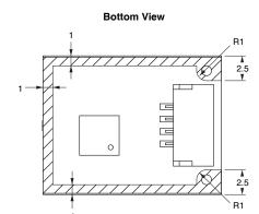
Note: Due to insulation distance limitations, do not allow metal parts to come into contact with the Sensor.
