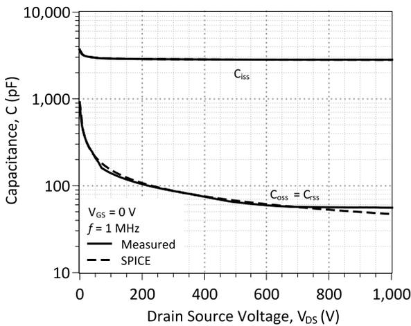
**Figure 9: Input, Output, and Reverse Transfer Capacitance**
