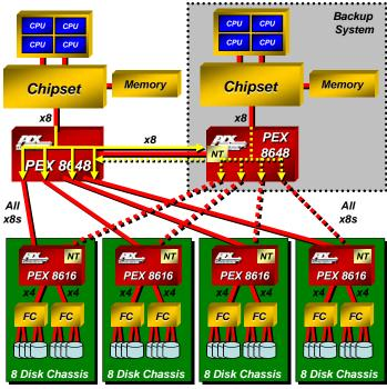
Figure 6. Dual Cast in Storage Systems
