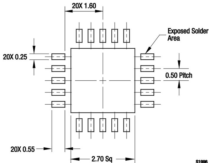
Figure 12. SKY13410-365LF PCB Layout Footprint (Top View)
