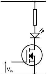
In this circuit an FET is connected to an LED, however it could be used to drive any load including higher power loads. When  $V_{in}$  is at zero volts the gate of the FET has no voltage on it, and no current flows through the LED. When  $V_{in}$  is high the FET turns on and current flows through the FET from the drain to the source and the LED lights.
