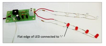
Current limit resistor for four LEDS 33Ω 3504 Standard red 3505 Standard green 33Ω 3506 Standard yellow 33Ω 3542 Standard white 220 3543 Standard blue 22Ω 3507 Ultra bright red 33Ω 3524 Ultra bright white 68Ω 3537 Ultra bright blue 68Ω
