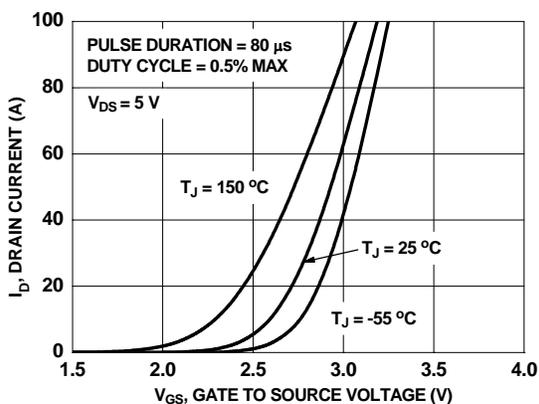
Figure 5. Transfer Characteristics
