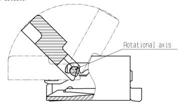
3. The actuator will not open more than 120°. Do not apply any force backward beyond this point. Otherwise, the actuator may come off or break.
