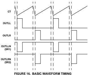
Referring to Figure 16, the SRs alternate between being both on during the free-wheeling portion of the cycle (OUTLL/LR off), and one or the other being off when OUTLL or OUTLR is on. If OUTLL is on, its corresponding SR must also be on, indicating that OUTLRN is the correct SR control signal. Likewise, if OUTLR is on, its corresponding SR must also be on, indicating that OUTLLN is the correct SR control signal.
