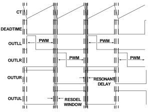
FIGURE 8. BRIDGE DRIVE SIGNAL TIMING
