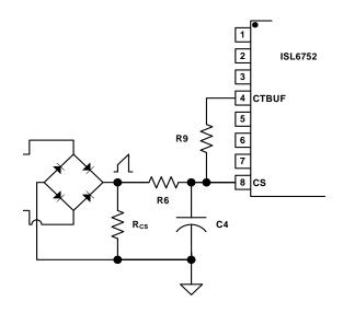
FIGURE 6. ADDING SLOPE COMPENSATION
