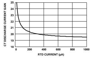
FIGURE 2. CT DISCHARGE CURRENT GAIN vs RTD CURRENT
