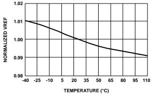
FIGURE 1. REFERENCE VOLTAGE vs TEMPERATURE
