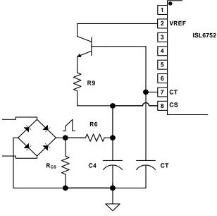
FIGURE 7. ADDING SLOPE COMPENSATION USING CT
