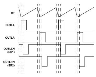
FIGURE 18. WAVEFORM TIMING WITH SR OUTPUTS DELAYED, 2.575V < VADJ < 5.00V
