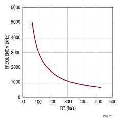
Figure 1. Switching Frequency vs RT
