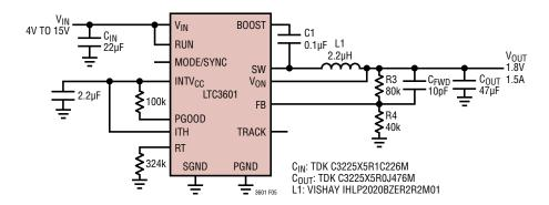
Figure 7. 1.8V, 1.5A Regulator at 1MHz
