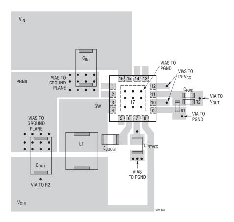
Figure 5. QFN Layout Example
