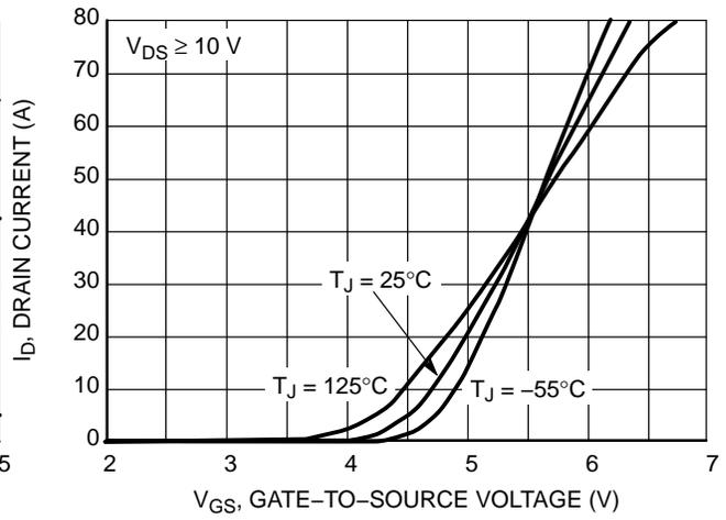
Figure 2. Transfer Characteristics
