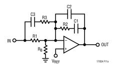
Figure 11a. Type 3 Amplifier Schematic Diagram
