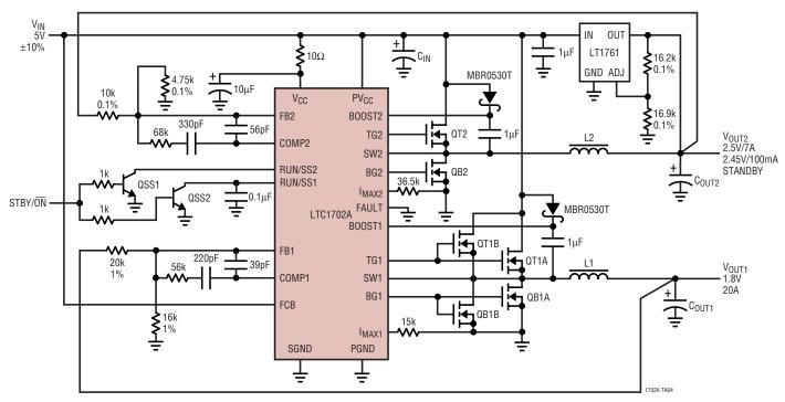
C<sub>IN</sub> = SANYO 10MV1200GX (6 IN PARALLEL) C<sub>OUT1</sub> = SANYO 6MV1500GX (8 IN PARALLEL) C<sub>OUT2</sub> = SANYO 6MV1500GX (3 IN PARALLEL) L1: 1μH SUMIDA CEP125-1R0MC-H
