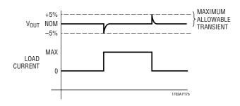
Figure 17b. Standard Regulator—Transient Response
