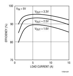
Figure 15. Typical LTC1702A Efficiency Curves
