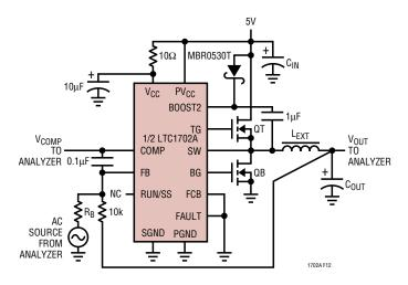
Figure 12. Modulator Gain/Phase Measurement Set-Up
