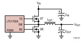
Figure 1. Synchronous Buck Architecture
