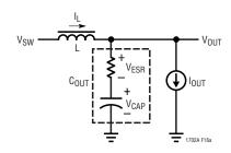
Figure 16a. Capacitor Parasitics Affecting Transient Recovery
