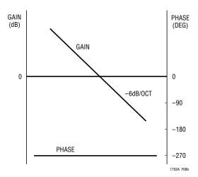
Figure 9b. Type 1 Amplifier Transfer Function
