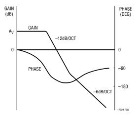
Figure 8. Transfer Function of Buck Modulator
