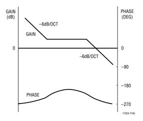
Figure 10b. Type 2 Amplifier Transfer Function
