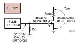
Figure 18. Transient Load Generator
