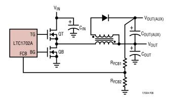
Figure 13. Regulating an Auxiliary Output with the FCB Pin
