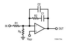
Figure 10a. Type 2 Amplifier Schematic Diagram
