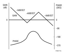
Figure 11B. Type 3 Amplifier Transfer Function
