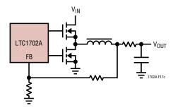
Figure 17c. Voltage Positioning Regulator
