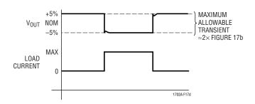
Figure 17d. Positioning Regulator—Transient Response
