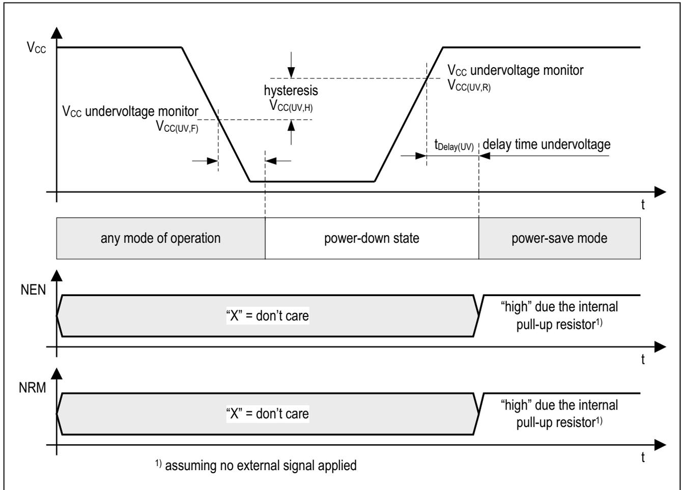
Figure 6 Undervoltage on the transmitter supply  $V_{CC}$
