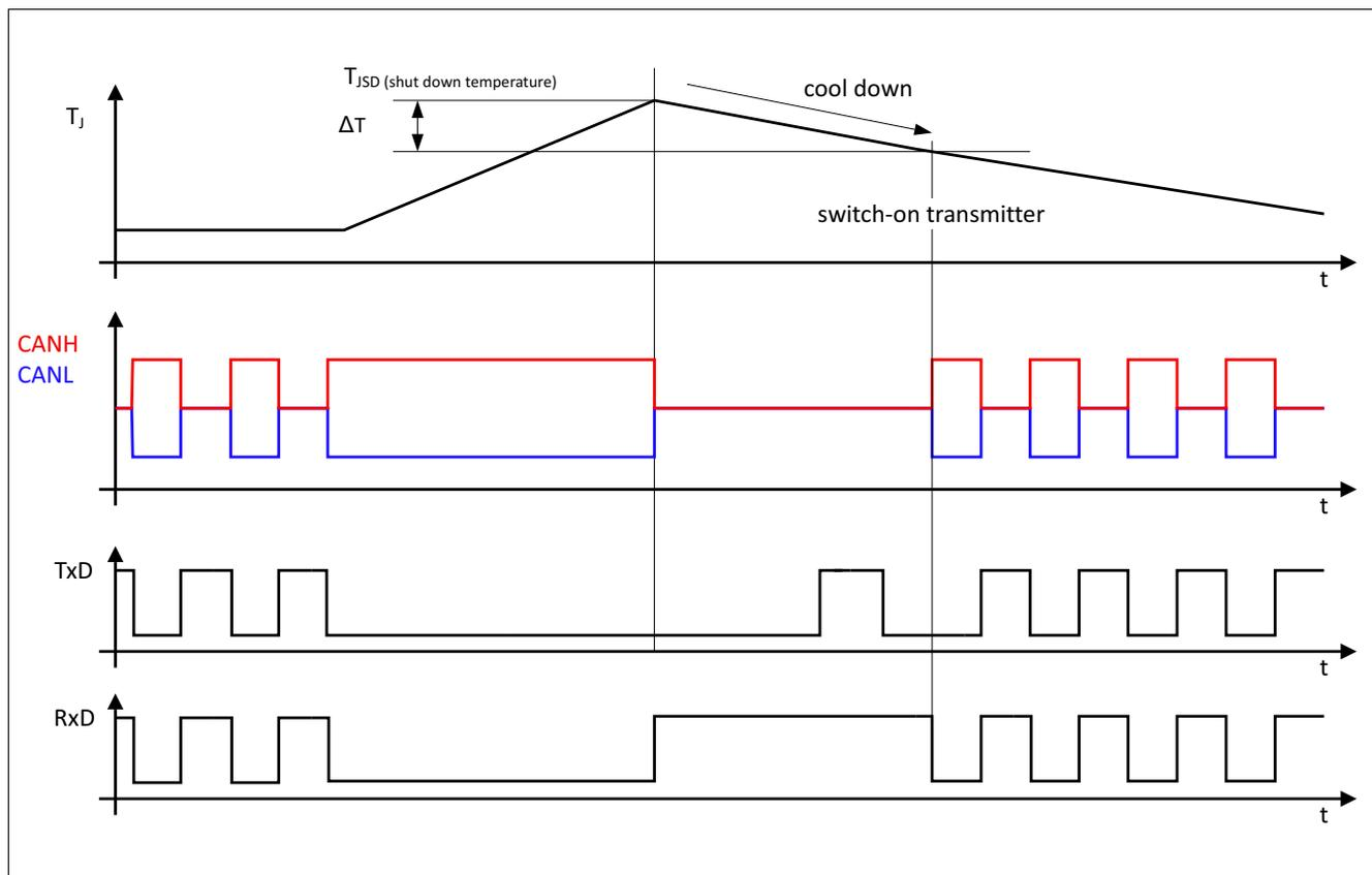
Figure 8 Overtemperature protection
