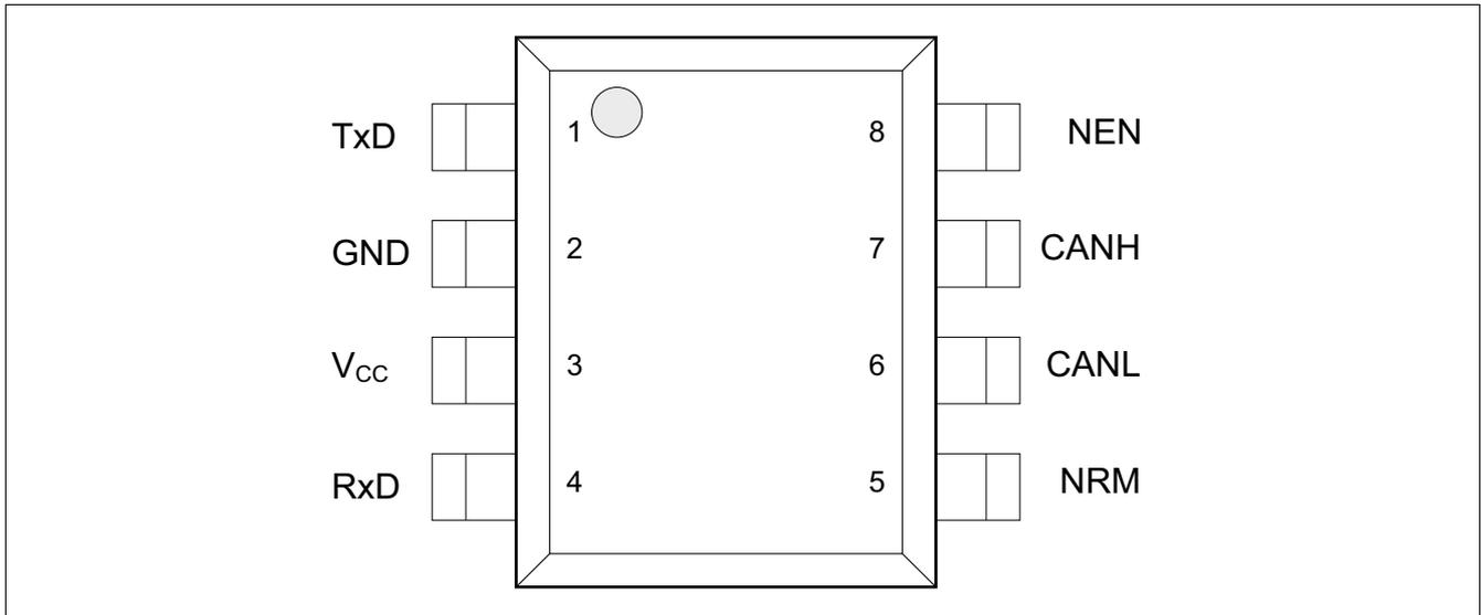
Figure 2 Pin configuration
