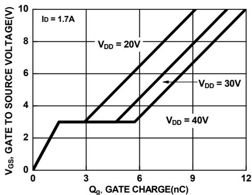
Figure 13. Gate Charge vs Gate to Source Voltage
