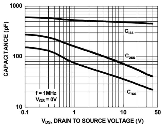
Figure 12. Capacitance vs Drain to Source Voltage
