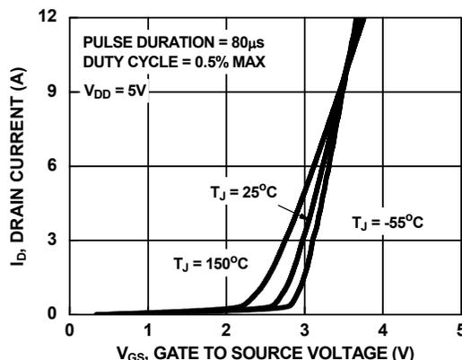
Figure 6. Transfer Characteristics
