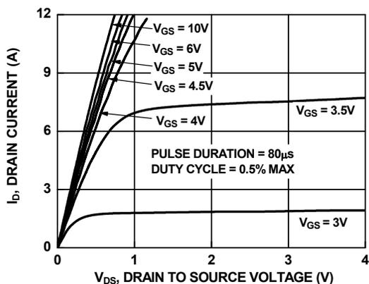
Figure 7. Saturation Characteristics
