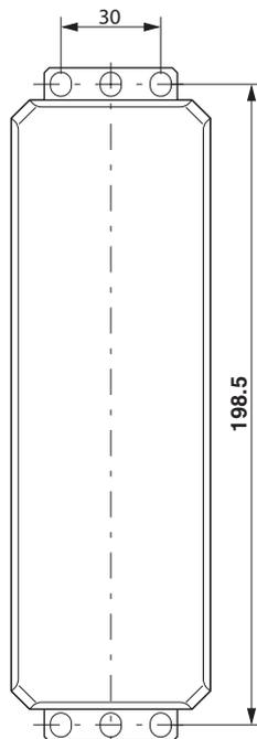
Figure 4-5 Drill hole spacing
