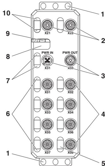
Figure 3-8 Basic structure of the Axioline E devices
