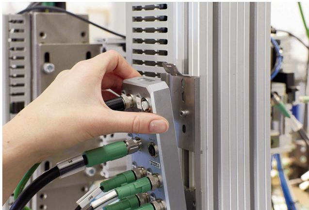
Figure 4-8 Snapping the metal device onto the mounting plate
