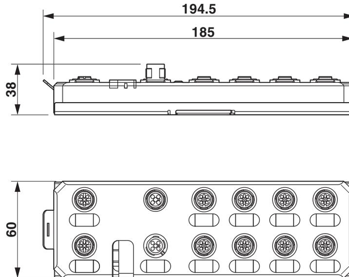
Figure 3-3 Housing dimensions (mm) of metal devices with mounting plate
