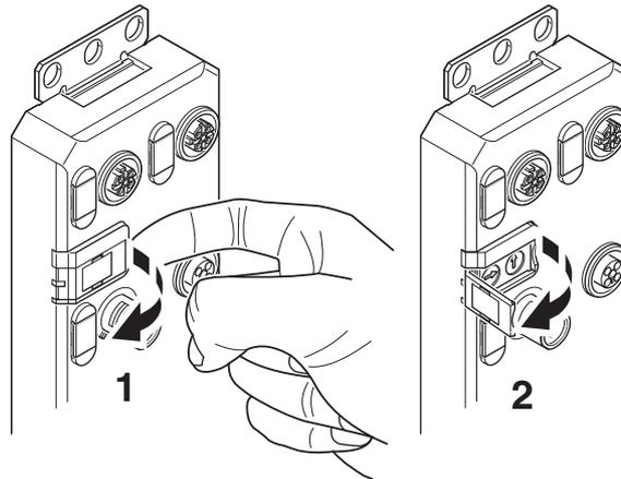
Figure 4-9 Opening the rotary coding switch cover
