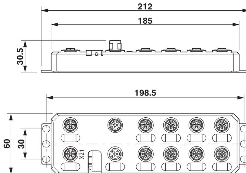
Figure 3-1 Housing dimensions (mm) plastic devices, Ethernet versions
