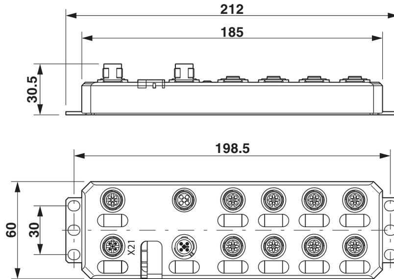
Figure 3-2 Housing dimensions (mm) of PROFIBUS plastic devices
