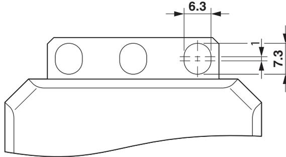
Figure 3-7 Dimensions of the screw holes in mm
