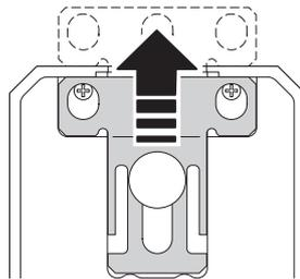
Figure 4-4 Extending the fixing clips of the metal device
