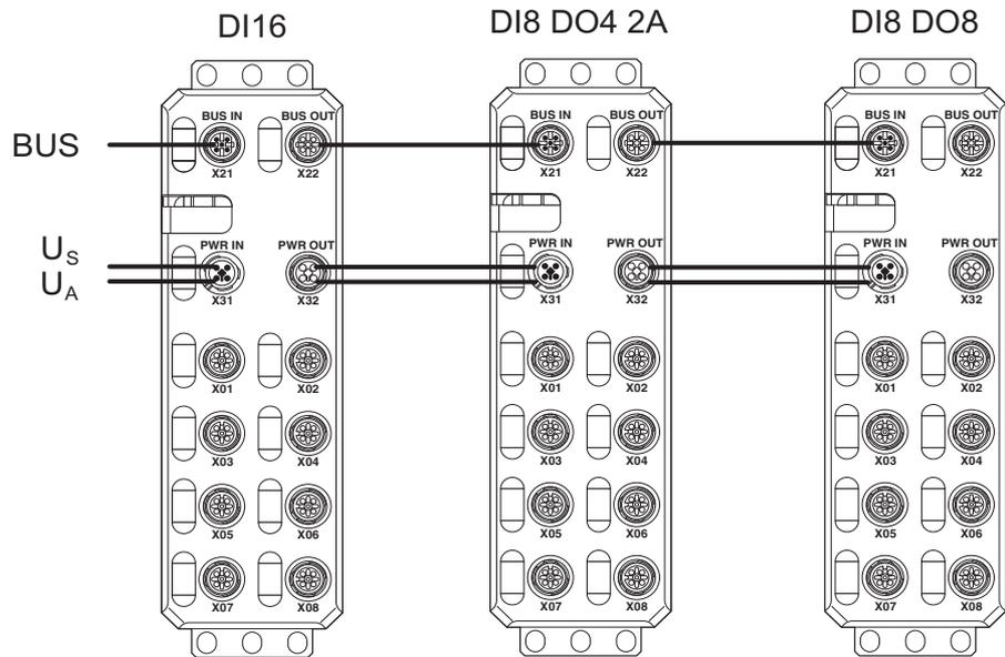
Figure 4-19 Example for the supply and forwarding of supply voltages
