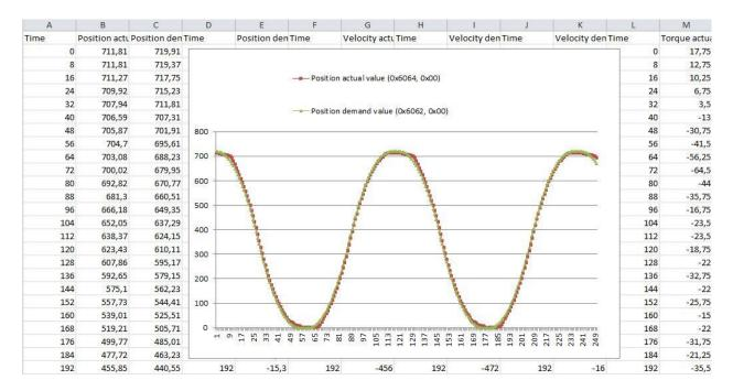
Notice that together with the channel description, you will find the internal register associated with this value. These registers are following the CANopen protocol structure since SMI21 CANopen drive is compliant with the following profiles: CiA-301, CiA-303, CiA-305, CiA-306 and CiA-402.
