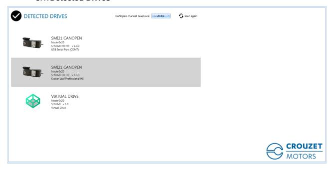
The **Drives** screen displays a list of the SMI21 CANopen drives that DCmind Soft + CANopen has found on your local network (CANopen or USB). You can select one of these drives from the list and click on the picture (grey line) to continue. This will connect you to the SMI21 CANopen drive and you will be given the option to use a wizard to setup the drive.
