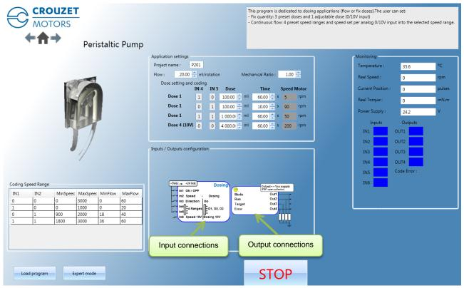
The "Peristaltic pump" application program uses a preset V201 expert program.
