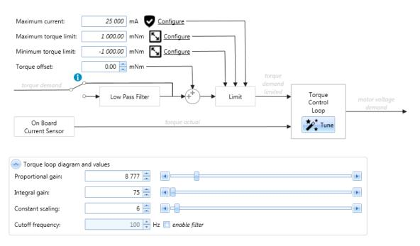
Max current parameter indicates the maximum permissible current creating torque in the motor.
