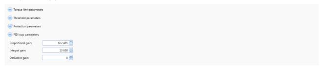
Set the PID controller factors in the speed control loop (this function is reserved for advanced users). The values given in the example below ensure correct product operation in the majority of cases.
