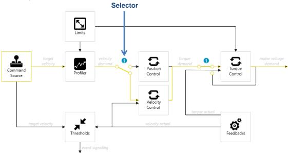
CAUTION: If your system is using a position sensor as a feedback (ex: encoder) it is highly recommended to use position loop for velocity modes.
