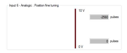
The motor position setpoint is the addition of position setpoint of IN5 and of position setpoint of IN6.
