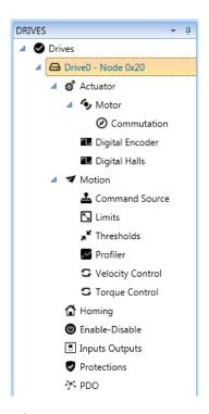
CAUTION: By default, only settings applicable to your current SMI21 CANopen drive operation mode, motor, feedbacks and command source will appear in this tree.
