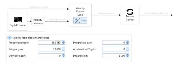
Note that you can set the position loop (or alternatively the velocity loop) for velocity modes such as homing or profile velocity with a selector:
