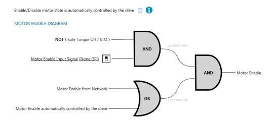
**Enable/Disable motor state is automatically controlled by the drive** parameter specifies if the motor should be automatically powered on (if possible) after power-up without the needed of user intervention.
