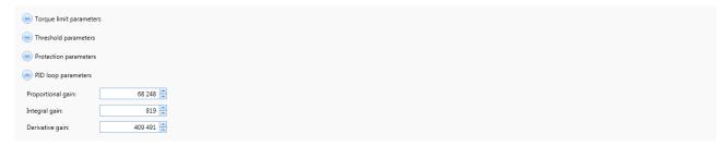
Set the PID controller factors in the position control loop (this function is reserved for advanced users). The values given in the example below ensure correct product operation in the majority of cases.
