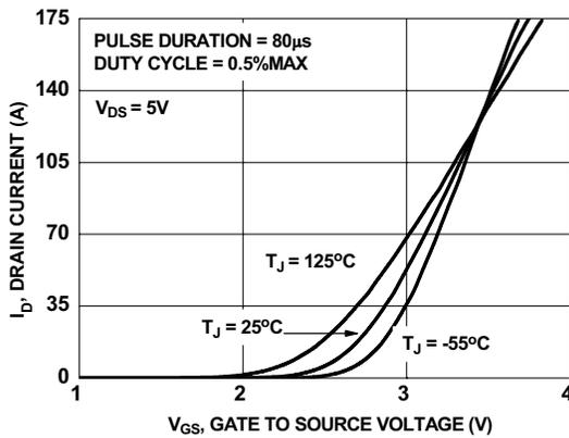
**Figure 5. Transfer Characteristics**
