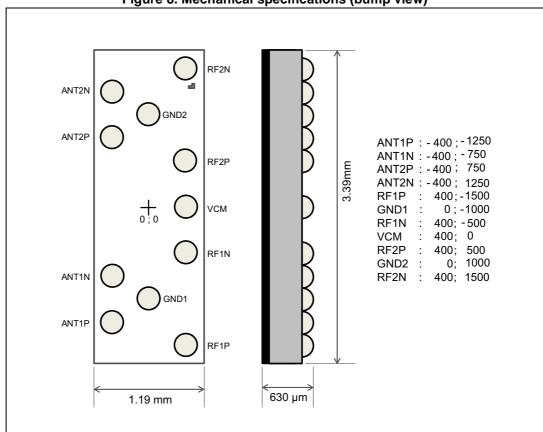
Figure 8. Mechanical specifications (bump view)
