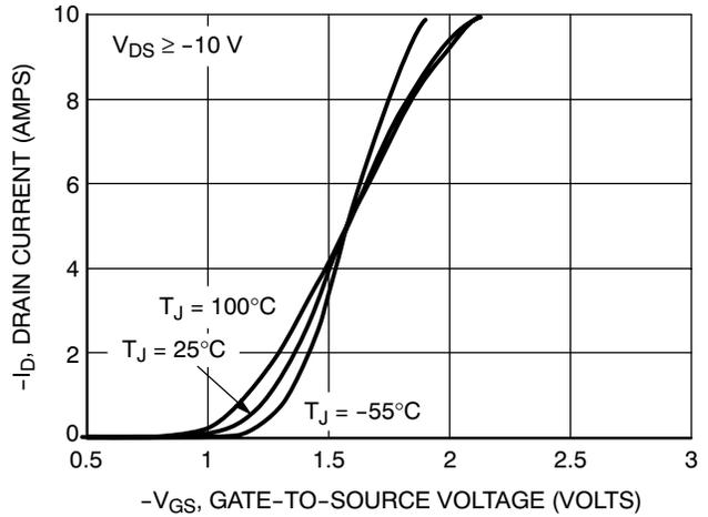
Figure 2. Transfer Characteristics
