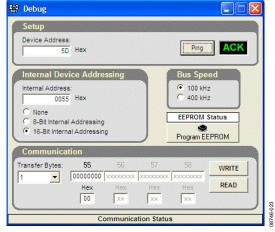
Figure 29. Evaluation Software I<sup>2</sup>C Debug Window
