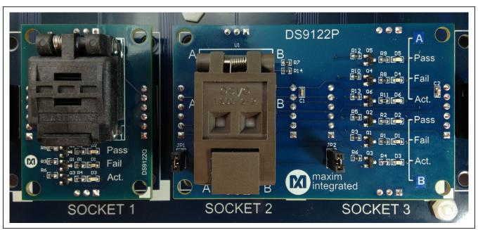
Figure 1. Single and Dual IC Socket Adapters
