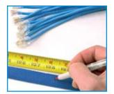
Measure the sleeving to length. Keep the sleeving relaxed and don't pull it as you measure. The most accurate method is to measure the sleeving on the actual application. There will be some foreshortening of the sleeving as it expands over large bundles or connectors. Mark the cut line with a pen or marker.
