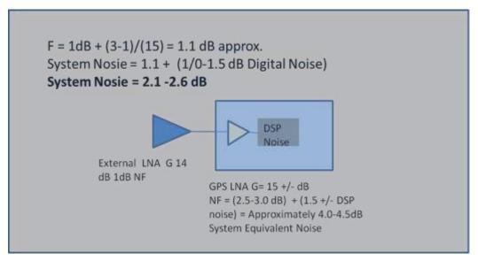
Figure 10-1 Cascade Noise Figure calculations with external LNA
