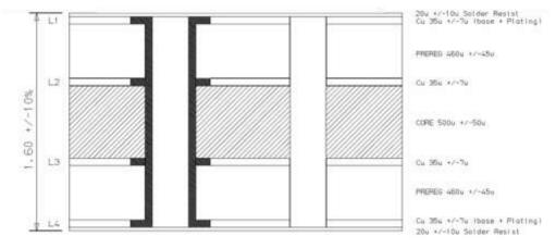
Figure 10-3 Example PCB Stackup
