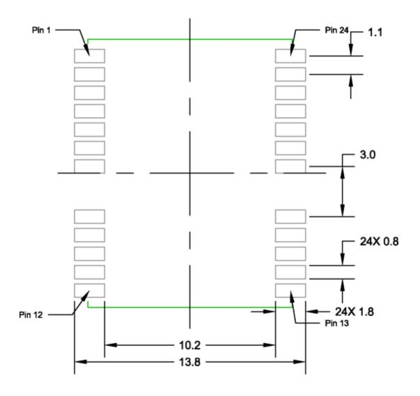
Figure 12-1 SL869 V2 and SL869 V2S PCB Footprint
