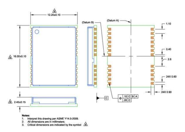
Figure 11-1 SL869 V2 and SL869 V2S Mechanical Drawing
