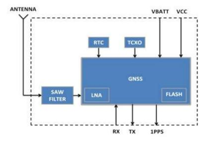
Figure 2-1 SL869 V2 Block diagram
