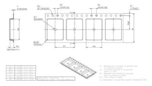
Figure 13-3 Tape and Reel Detail
