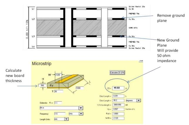
Figure 10-5 Example of wider trace width achieved by moving ground plane
