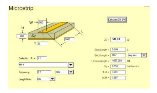
Figure 10-4 Typical Board stackup and calculated trace width
