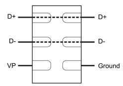
Figure 2. Flow-through Layout
