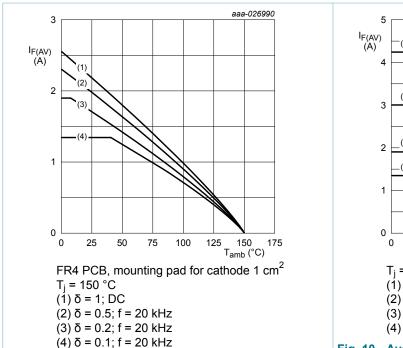
Fig. 9. Average forward current as a function of ambient temperature; typical values
