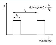
Fig. 14. Duty cycle definition
