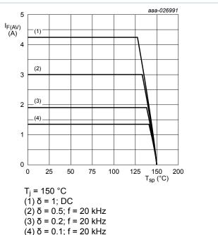
Fig. 10. Average forward current as a function of solder point temperature; typical values
