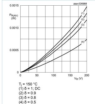
Fig. 7. Average reverse power dissipation as a function of reverse voltage; typical values
