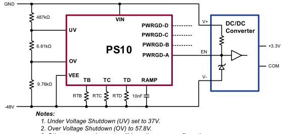
3. Other power good outputs will have the same configuration as PWGRGD-A for Active High Enabled Converters.
