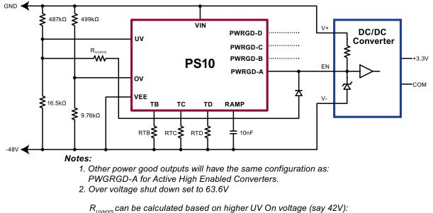
$\begin{aligned} & \mathcal{R}_{UVHYS} \text{ can be calculated based on higher of V On Voltage (say 42V).} \\ & \mathcal{R}_{UVHYS} = (V_{UVON} - V_{DIODE} - V_{PWRGDLOW}) / ((V_{IN} - V_{UVON}) / 487k\Omega - V_{UVON} / 16.5k\Omega) \\ &= (1.22 - 0.65 - 0.4) / ((42 - 1.22) / 487k\Omega - 1.22 / 16.5k\Omega) \\ &= 17.35k\Omega \end{aligned}$
