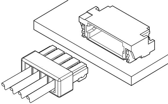
**This SUH connector is developed for crimping type SUR connector that has been designed for 0.8 mm pitch wire-to-board insulation displacement connector. This connector adopted the first crimping method in a minimum 0.8 mm pitch of the wire-to-board type connector. Housing lance method provides the good workability and a constriction contact method provides the excellent contact reliability.**
