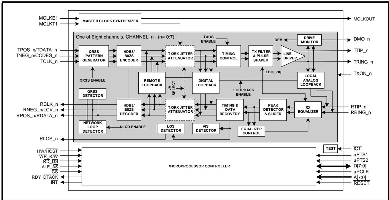
FIGURE 2. BLOCK DIAGRAM OF THE XRT83L38 T1/E1/J1 LIU (HARDWARE MODE)
