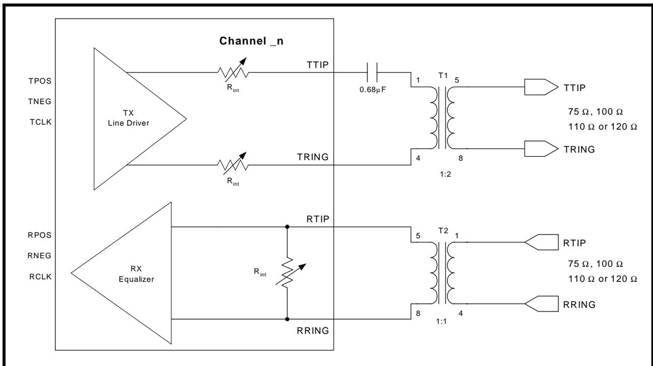
If the internal termination mode (RXTSEL = “1”) is selected, the effective impedance for E1, T1 or J1 can be achieved either with an internal resistor or a combination of internal and external resistors as shown in Table 7.
