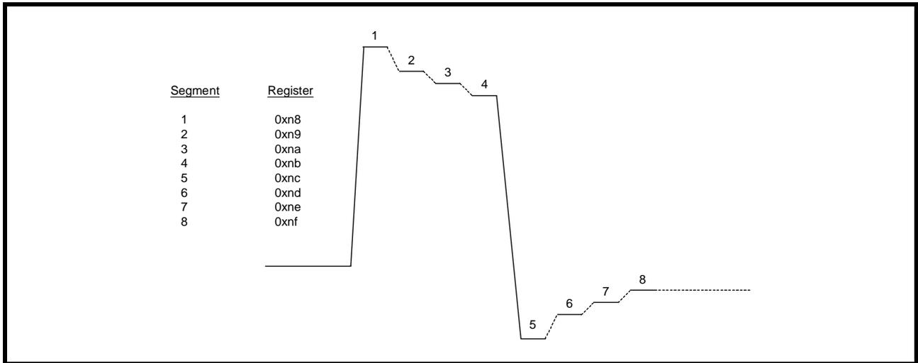
**NOTE:** By default, the arbitrary segments are programmed to 0x00h. The transmitter outputs will result in an all zero pattern to the line. For E1 arbitrary mode, see global register 0xC0h.
