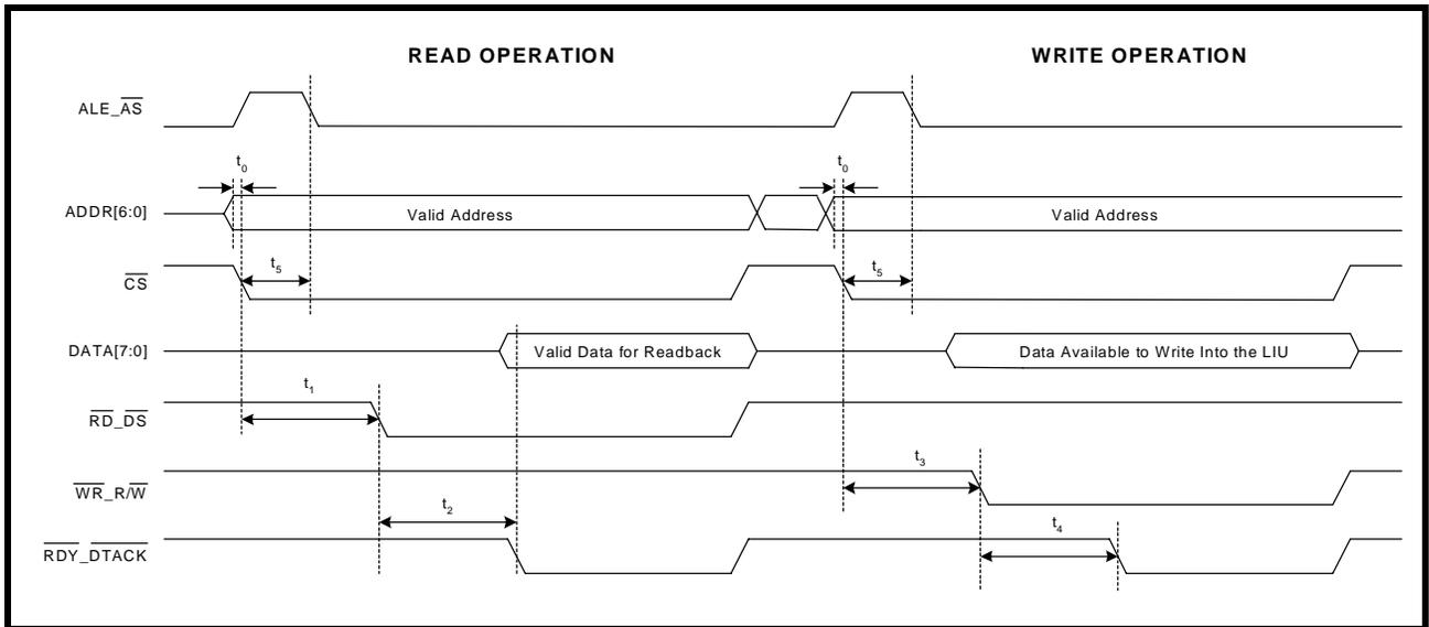
TABLE 51: ASYNCHRONOUS MODE 1 - INTEL 8051 AND 80188 INTERFACE TIMING
