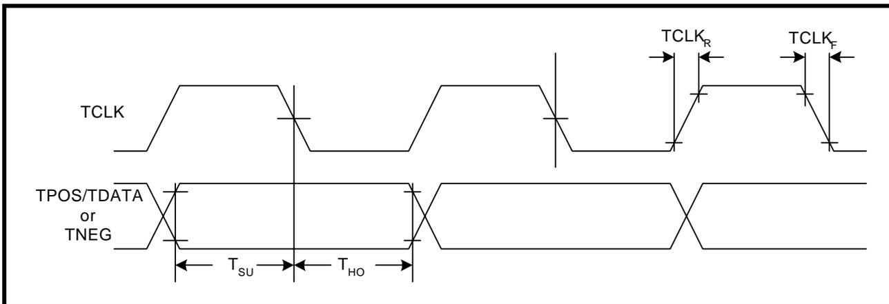
**FIGURE 29. RECEIVE CLOCK AND OUTPUT DATA TIMING**
