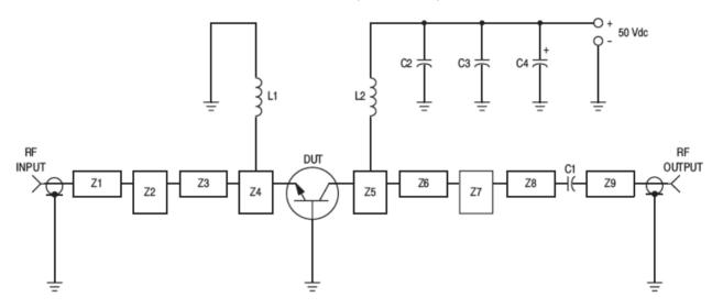
C1, C2 — 220 pF Chip Capacitor, 100–mil ATC C3 — 0.1 μF C4 — 47 μF/75 V L1, L2 — 3 Turns #18 AWG, 1/8″ ID
