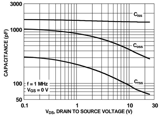
**Figure 8. Capacitance vs Drain to Source Voltage**
