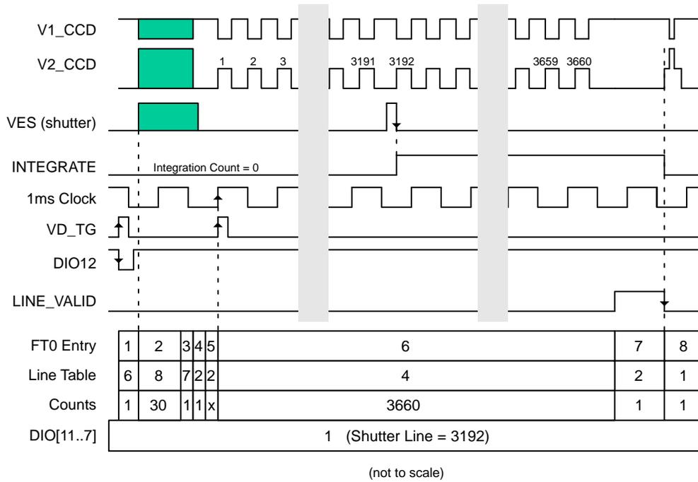
Figure 27. Still Mode Integration Timing with Shutter
