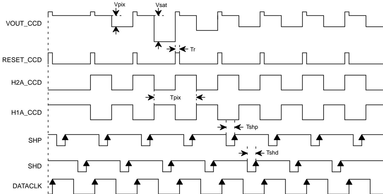
**Figure 20. Horizontal Timing**
