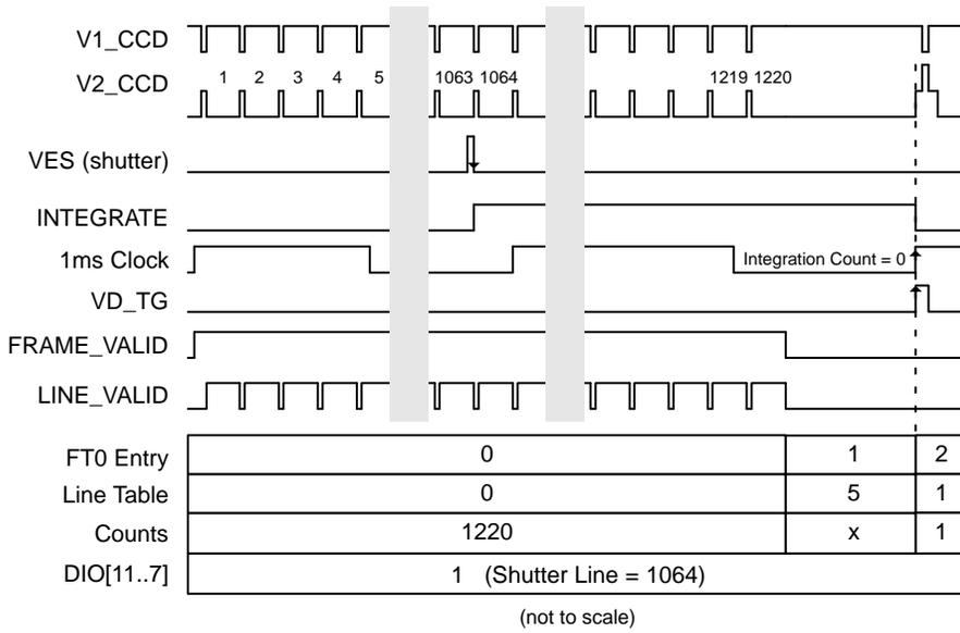
**Figure 24. Free-Running Mode Integration Timing with Shutter**
