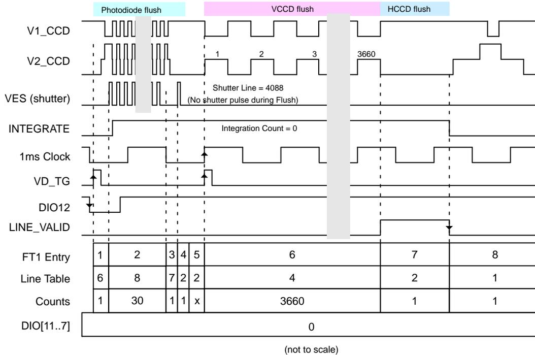
**Figure 26. Still Capture Mode Default Integration Timing**
