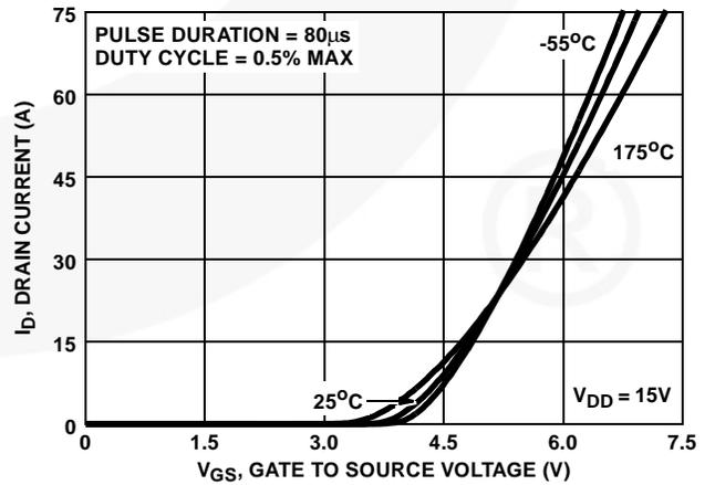
FIGURE 8. TRANSFER CHARACTERISTICS
