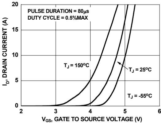
Figure 5. Transfer Characteristics
