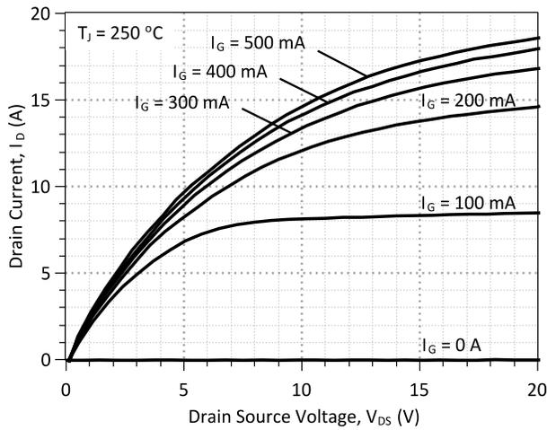
Figure 3: Typical Output Characteristics at 250 °C
