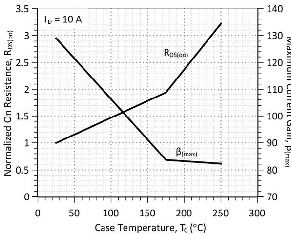
Figure 5: Normalized On-Resistance and Current Gain vs. Temperature
