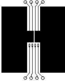
a) 78 $^{\circ}\text{C}/\text{W}$  when mounted on a 0.5in<sup>2</sup> pad of 2 oz copper
