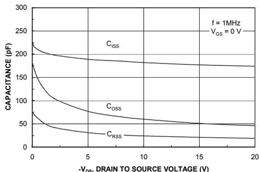
Figure 8. Capacitance Characteristics.
