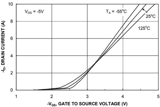
**Figure 5. Transfer Characteristics.**
