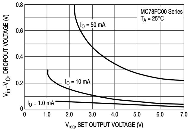
Figure 2. Dropout versus Set Output Voltage
