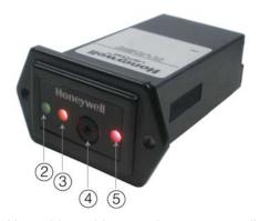
NOTE: Use a blunt object, such as a paper clip or tooth pick to actuate the function switch 4.
