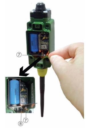
NOTE: Use a blunt object, such as a paper clip or tooth pick to actuate the function switch  $\ensuremath{\mathfrak{D}}.$
