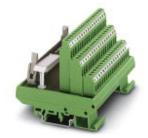
VARIOFACE module, with screw connection and flat-ribbon cable connector, for mounting on NS 32 or NS 35/7.5, with pin strip and short and long locking latches for socket strips, 50-pos.
