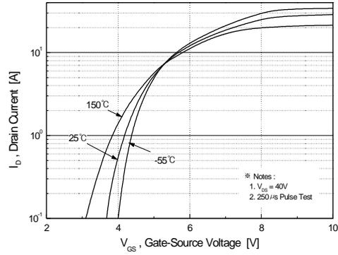
Figure 2. Transfer Characteristics
