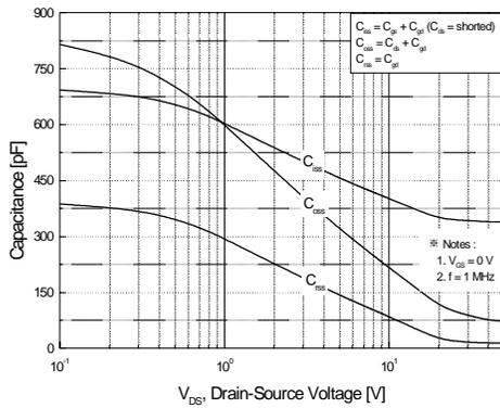
Figure 5. Capacitance Characteristics
