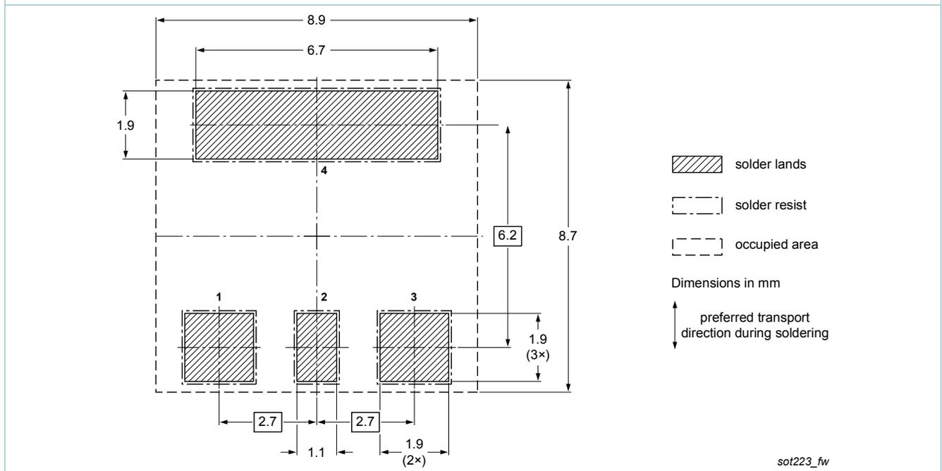
Fig. 20. Wave soldering footprint for SC-73 (SOT223)
