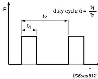
Fig. 17. Duty cycle definition
