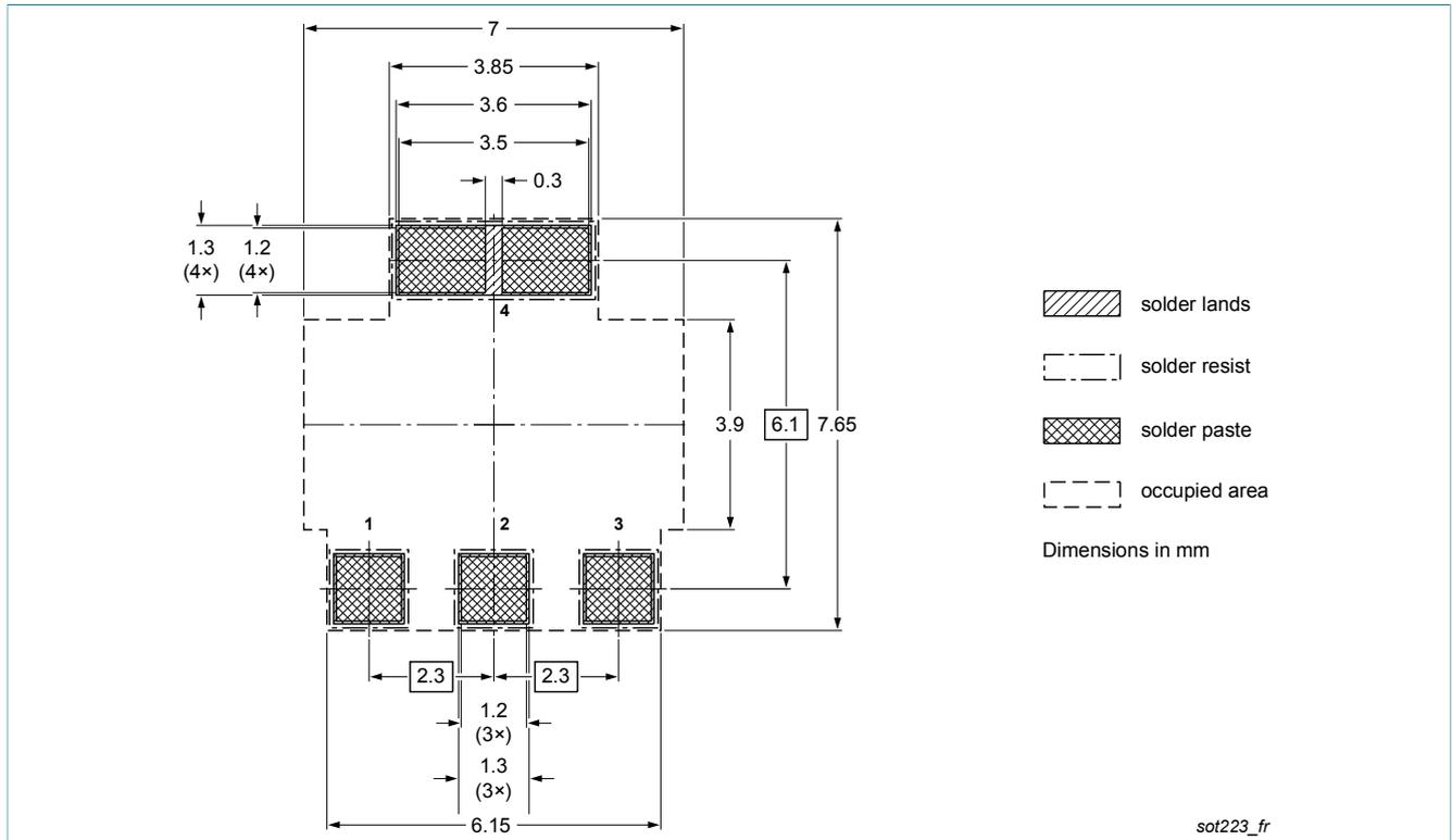
Fig. 19. Reflow soldering footprint for SC-73 (SOT223)
