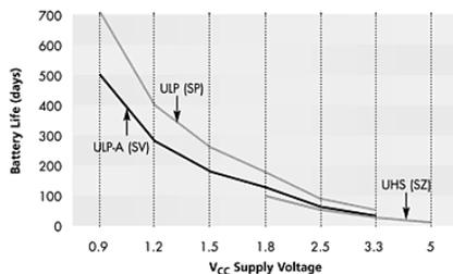
TinyLogic ULP and ULP-A with up to 50% less power consumption can extend your battery life significantly.
