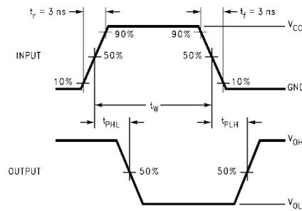
FIGURE 2. AC Waveforms
