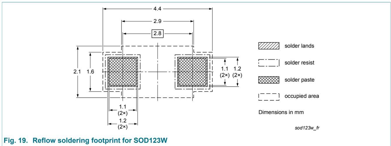
Fig. 19. Reflow soldering footprint for SOD123W
