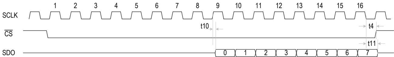
**Figure-35 Serial Interface Read Timing with CLKE = 0**
