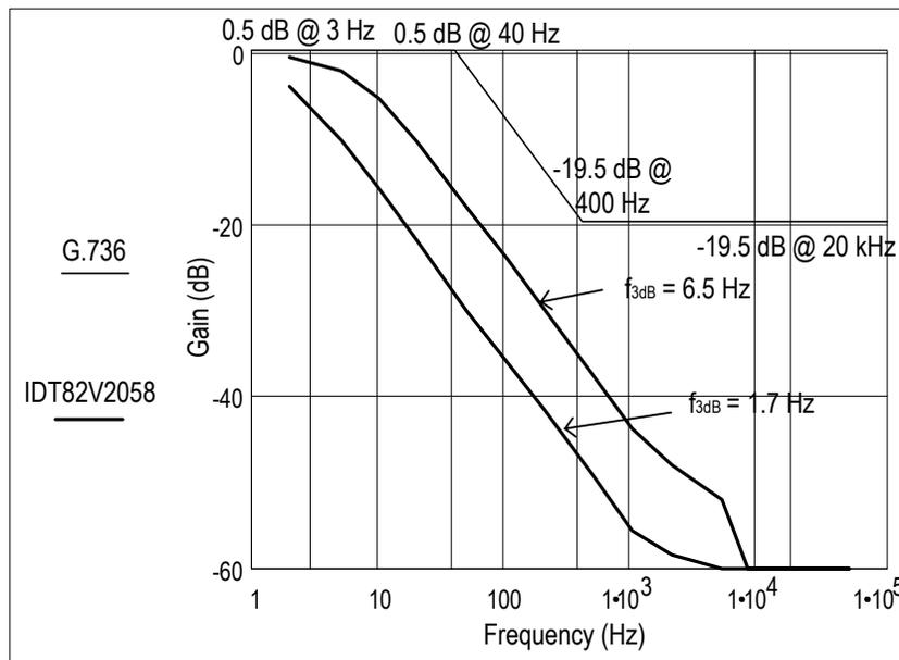
Test condition: PRBS 2<sup>15</sup>-1; Line code rule HDB3 is used.
