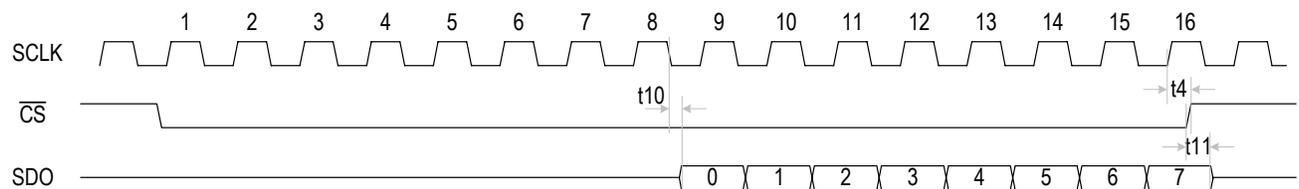
**Figure-36 Serial Interface Read Timing with CLKE = 1**
