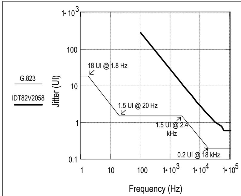
Test condition: PRBS 2<sup>15</sup>-1; Line code rule HDB3 is used.
