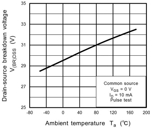
**Fig. 8.7  $V_{(BR)DSS} - T_a$**
