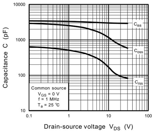
**Fig. 8.11 Capacitance -  $V_{DS}$**
