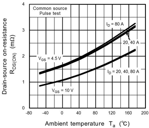
**Fig. 8.9  $R_{DS(ON)} - T_a$**
